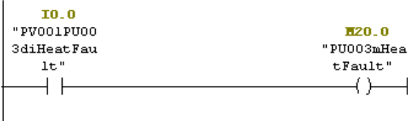
Figure 9 - Digital input mapping to a Memory Address in a Siemens PLC
