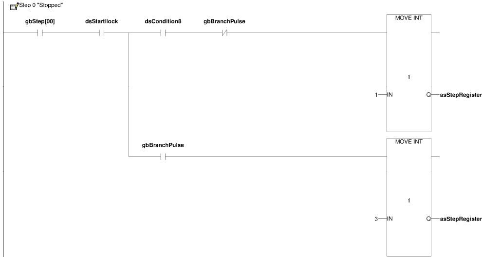
Figure 19 - Typical logic for sequence step of GE PLC
