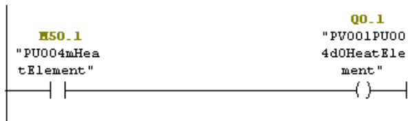
Figure 10 - Mapping a Memory Address to a digital output in a Siemens PLC
