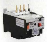
The CT 4 is fitted with a built-in wire connection to provide a series connection between its trip contact and the 'A2' coil termination of a contactor. This connection can be removed if not required.
