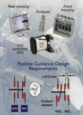
CS 4 control relays are perfect for fail-safe control circuits. An interlock contact design, which maintains minimum 0.3 mm clearance, prevents the N/C contacts from reclosing if the N/O contact is welded when in operation. (This feature includes the base contact poles only and does not extend to the front mounted auxiliary contacts).
