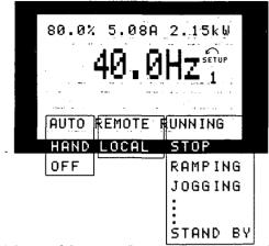
The left part of the status line indicates the control element of the VLT frequency converter that is active.
