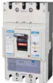
**Trip unit:** Fixed thermal, adjustable magnetic 6 x 12 li**Earth leakage characteristic:** Type "AC" - suitable for AC currents.**Earth leakage adjustments:** 100 mA, 200 mA, 500 mA
