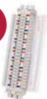
The Concept range of busbar chassis assemblies have been specifically designed for incorporation into the Concept family of panelboards, providing a secure mounting platform and connection system for the NHP Din-T range of MCBs. The busbars are fully enclosed therefore not requiring an insulated coating for electrical isolation. The new GB chassis has an isolation switch for each individual TEE-OFF, are type tested and are mounted on a box section steel pan, powdercoated white.
