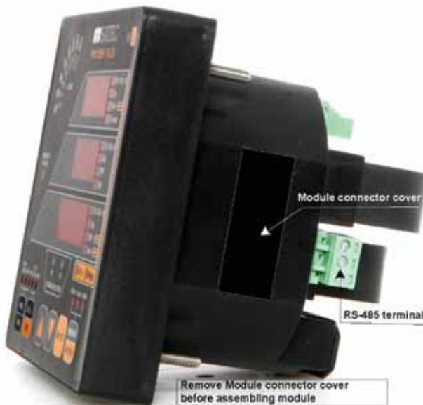
Figure 2-17 Module Connector Cover – Before Module Assembly
