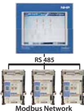
**Notes:** <sup>1)</sup> ACBs must be fitted with a remote tripping device and charging motor. For TemVision Pro information, refer to NHP.
