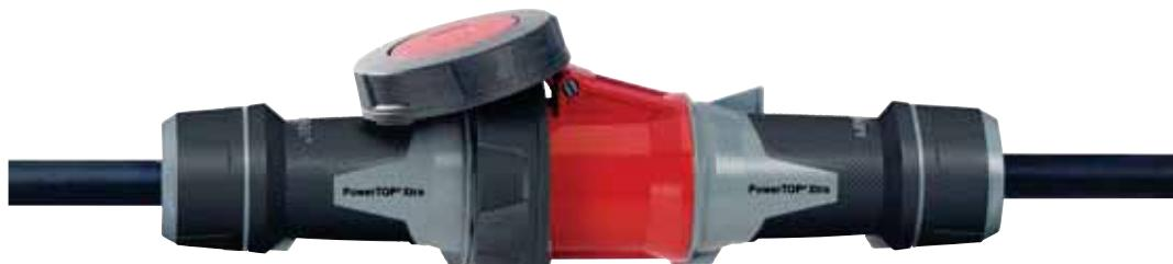
**PowerTOP Xtra** is rubberized for the best grip. Improved impact resistance even under humid conditions. Highly heat-resistant contact carrier, frame terminals, cable gland and sealing, strain relief and protection against kinking. Enclosure with thread lock, two safety slides and plugs with nickel-plated contacts. Connectors 63A with **SoftCONTACT** and 125A with **TorsionSpringCONTACT**.
