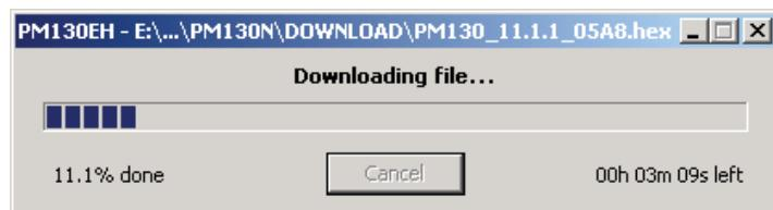
7. After upgrading firmware is completed, the meter restarts, so communications can be temporarily lost. You may need to wait a short duration until PAS restores a connection with your device.
