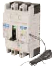
**3****Trip unit:** Adjustable thermal (0.63 I<sub>r</sub> to 100 % I<sub>r</sub>) and fixed magnetic**Earth leakage characteristic:** Type 'A' - suitable for AC and residual pulsating DC currents.**Earth leakage adjustments:** - 30 mA, 100 mA, 300 mA, 500 mA, 1 A, 3 A.
