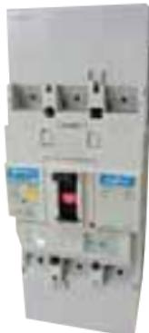
**Trip unit:****Adjustable thermal:** 63% Ir to 100% Ir**Adjustable magnetic:**  $6 \times I_m$  to  $13 \times I_m$  for 160 A trip unit types $6 \times I_m$  to  $10 \times I_m$  for 250 A trip unit types**Dimensions (mm)**
