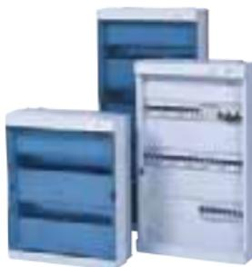
These enclosures have generous 150 mm wiring space between and 30 mm behind equipment rails. The removable mounting frame serves to ease cabling and wiring greatly. Din-Modula 150 is designed for indoor use and to accept the Din-T 6, 10, 10H and 15 MCB range, time switches, contactors and main switches.
