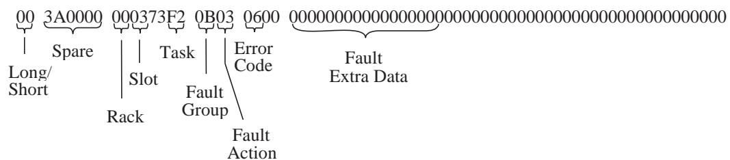
This System Configuration Mismatch fault entry is explained below. (All data is in hexadecimal.)
