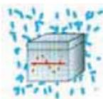
Protected against water sprayed from all directions - limited ingress permissible.
