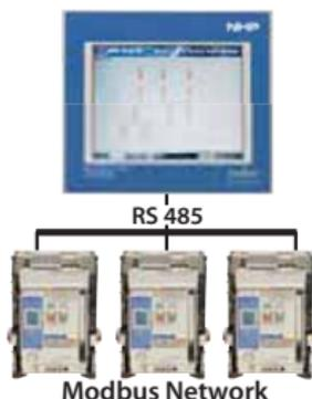
**Notes:** <sup>1)</sup> ACBs must be fitted with a remote tripping device and charging motor. For TemVision Pro information, refer to NHP.
