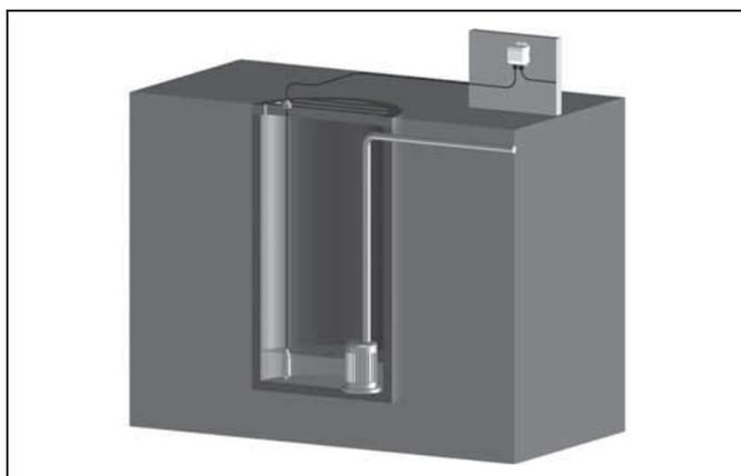
Fig. 3: VEGAWELL 52 in a pump shaft with VEGABOX 02
