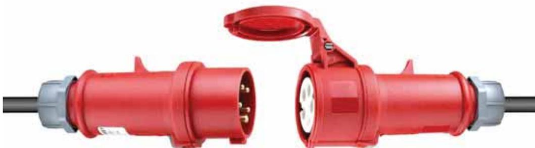
with SafeCONTACT, screwless with insulation displacement technique, cable gland with sealing, strain relief and protection against kinking, 2-part enclosure with thread lock and safety slider.
