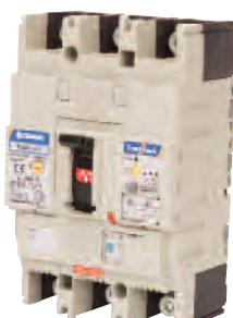
The ZS earth leakage ELCB from Terasaki offers machine or personnel protection within a standard 125 A, 160/250 A MCCB frame size. The ZS earth leakage ELCB also maintains the full functionality of a standard thermal-magnetic overload / short circuit protection device.
