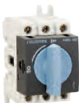
The SIRCO M range of load-break switches offer compact IP 20 finger safe solutions for switching up to and including 125 A. They are ideal for the arduous switching of motors.
