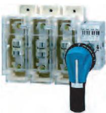
SSF Standard switch-fuses boast IP 30 protection on all fuse terminals in a compact yet effective design. These switch-fuses feature a test position and double-break contacts per phase, allowing the safe isolation of AC and DC circuits as well as the added short circuit protection offered by HRC fuses.
