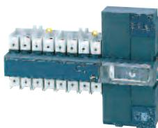
The ATyS M 3s is made up of 2 power switches that are mechanically and electrically interlocked to ensure safe operation. The 3s is driven by a volt free contact allowing switching operation between I, 0, II from external control logic. The 3s features solenoid operation to ensure fast switching operations. ATyS M 3s Transfer switches require external control for switching and or circuit sensing.
