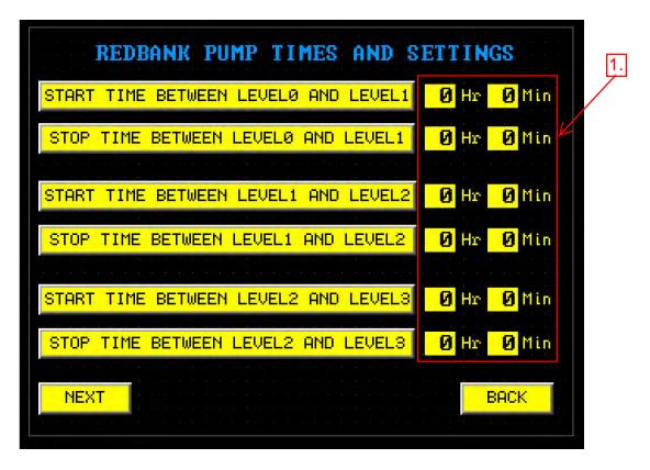
The Redbank Pump Times screen displays the restriction times applied to the Redbank Pump for each Detention Tank level.
