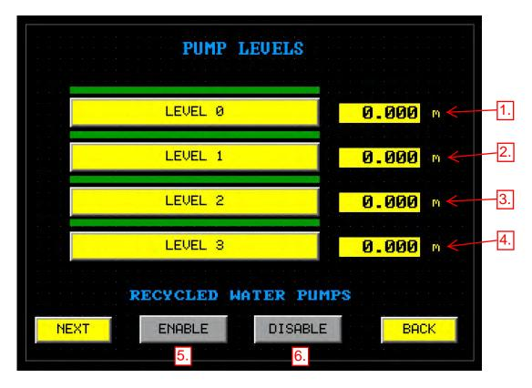
The Recycled Water Pump Restriction Levels screen displays the Chlorine Detention Tank levels for each time based restriction applied to the Recycled Water supply pumps. There are four (4) level set points that are displayed in m. above sea level. The lower the level in the Detention Tank the more time based restrictions are applied to the Recycled Water supply pumps.
