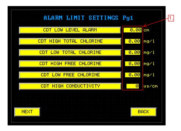
The Alarm Limit Settings Page 1 screen is used to adjust the alarm limit settings for the Detention Tank Effluent levels, Chlorine levels and Conductivity levels.
