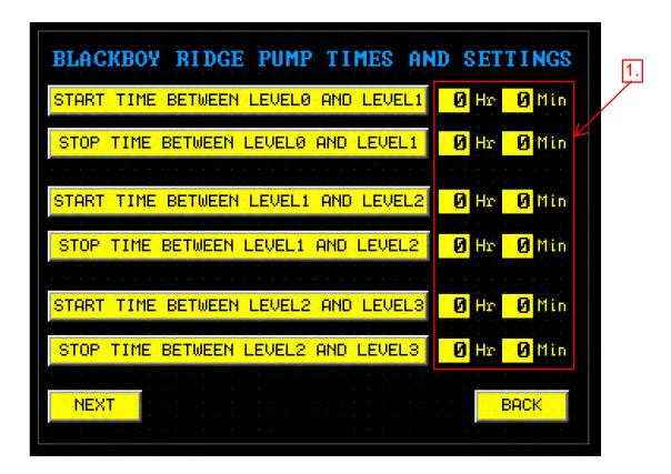
The Blackboy Ridge Pump Times screen displays the restriction times applied to the Blackboy Ridge Pump for each Detention Tank level.
