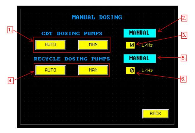
The Manual Dosing screen is used to select automatic or manual dosing for the Detention Tank and Recycled Water dosing pumps.
