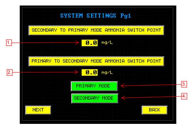
The System Settings Page 1 screen controls the set points for automatic switching between Primary Mode and Secondary Mode dosing.
