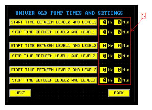
The University of Queensland Pump Times screen displays the restriction times applied to the University of Queensland Pump for each Detention Tank level.
