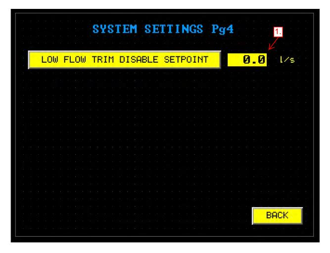
The System Settings Page 4 screen controls the "Low Flow Trim Disable Set Point" which prevents the control system dosing under Trim Dosing if water flow is below the set point.
