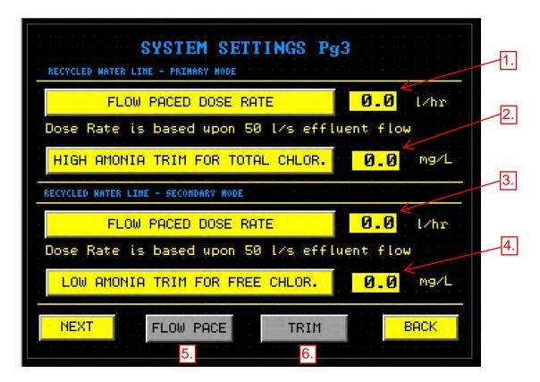
The System Settings Page 3 screen controls the dose rate into the Recycled Water Pipe that supplies recycled water to the customer supply pumps.
