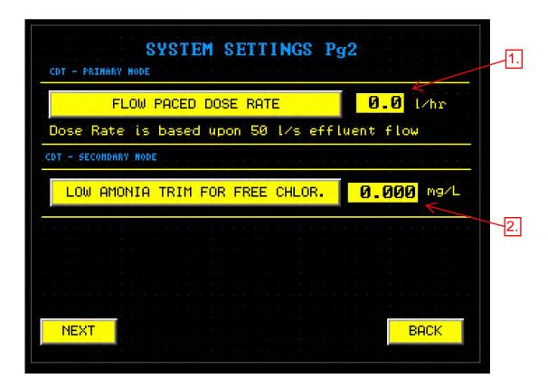
The System Settings Page 2 screen controls the dose rate into the Detention Tank.
