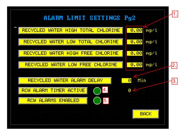
The Alarm Limit Settings Page 2 screen is used to adjust the alarm limit settings for the Recycled Water Chlorine levels.
