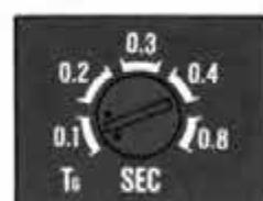
The GFT has a definite time-delay characteristic, its opening time is adjustable from; 100, 200, 300, 400 to 800ms
