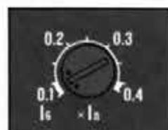
The GFT pick-up current ( $I_s$ ) is continuously adjustable from 10% to 40% of the rated current ( $I_o$ ).
