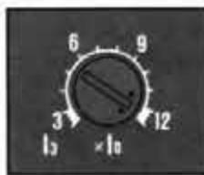
The INST pick-up current ( $I_o$ ) is continuously adjustable from 300% to 1200% of the rated current ( $I_o$ )
