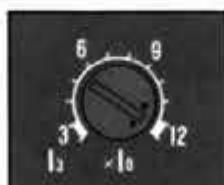
The INST pick-up current ( $I_s$ ) is continuously adjustable from 300% to 1200% of the rated current ( $I_o$ ).
