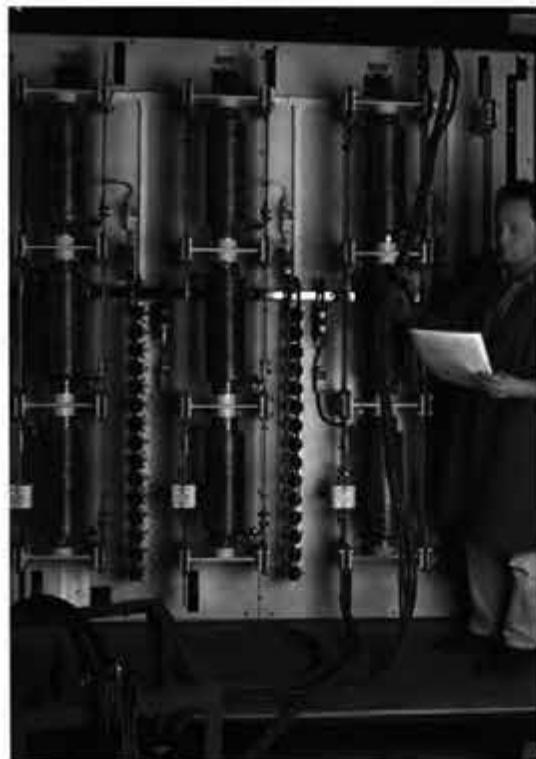
**FIGURE 7.** Critec maintains a fully equipped High Voltage Test Laboratory. All product designs are extensively tested for surge handling capability, design optimisation and load performance. Seen above, a three phase Proline 1600A SRF under going full load current tests and burn in test cycles.
