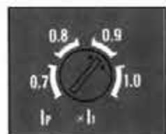
The PTA pick-up current ( $I_o$ ) is adjustable from 70, 80, 90 to 100% of the rated current ( $I_o$ ). The time-delay is 40 seconds fixed. (A separate power source is required)
