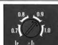
The PTA pick-up current ( $I_s$ ) is adjustable from 70, 80, 90 to 100% of the rated current ( $I_o$ ). The time-delay is 40 seconds fixed. (A separate power source is required)
