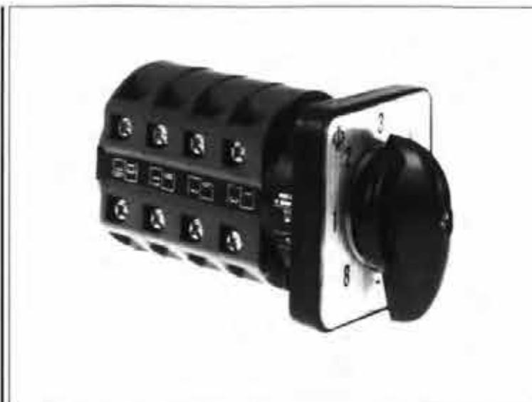
The terminals of the CA series cam switches are accessible from both sides. This is an advantage in cases where the switch is prewired for installation or in cases where the terminal wiring cannot be done in the sequence of the stage. The compact design, the excellent switching capabilities under AC11, AC3 and AC23 and the obviously unlimited number of switch developments are characteristic for the CA switches.
