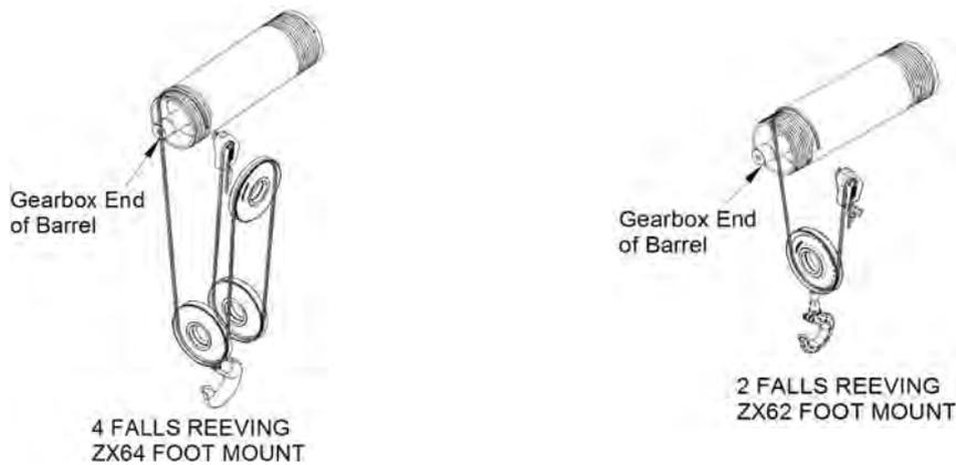
Figure 55 – Reeving Diagrams for Foot Mount Hoists: ZX062-FTM / ZX064-FTM
