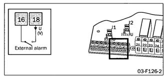
Fig. 66 Connection of terminals for external alarm
