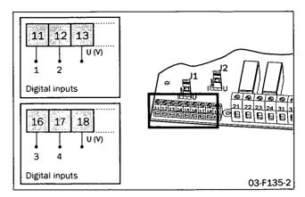
Fig. 57 Wiring for digital inputs 1-4.
