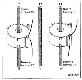
Fig. 50 Current transformer position for Bypass on MSF-017 to MSF-250.
