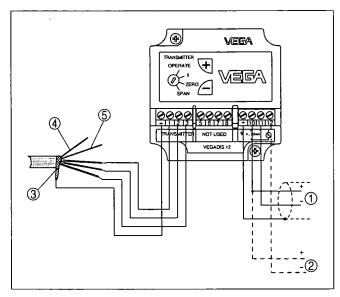
Fig. 6: Terminal assignment, VEGADIS 12
