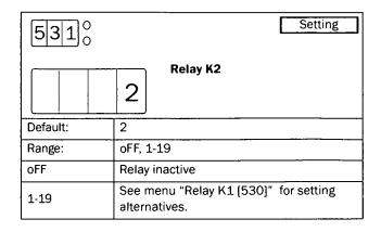
NOTE: If relay K2 is chosen to be inactive (oFF), the relay state is determined by the contact function in menu [534].
