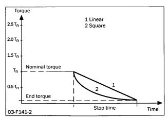
Fig. 43 Torque control at stop
