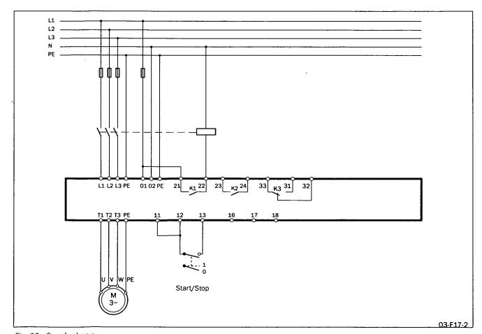
Fig. 25 Standard wiring.
