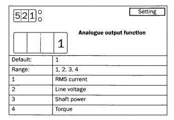
The scaling of the analogue output is reset to the default values (0-100%) if a new output value is chosen in menu [521].
