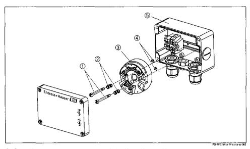
Fig. 7: Mounting the temperature transmitter, depicted here with terminal box Only open terminal box with a screwdriver.
