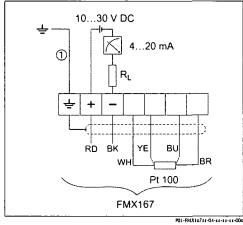
FMX167 electrical connection, versions "7" or Fig. 8: "3" for Feature 70 "Additional options" in the
