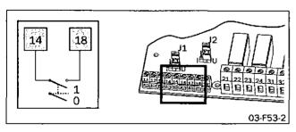
Fig. 54 Wiring for digital input signal.
