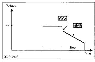
Fig. 44 Menu numbers for step down voltage at stop and stop time.
