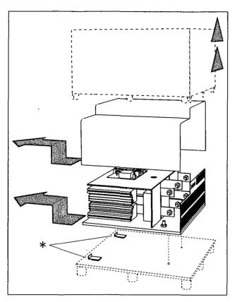
Fig. 2 Unpacking MSF-310 and larger models.
