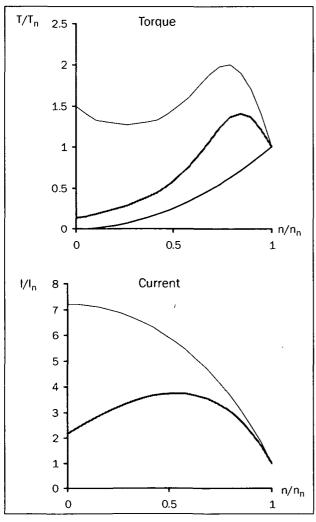
Fig. 8 Soft starting - voltage ramp
