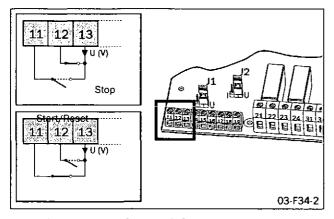
Fig. 64 Connection of terminals for start/stop/reset
