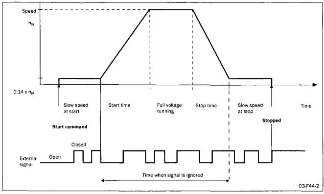
Fig. 46 Slow speed controlled by an external signal.
