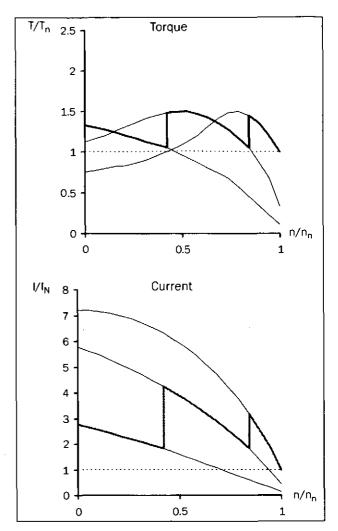
Fig. 11 Rotor-resistance starting
