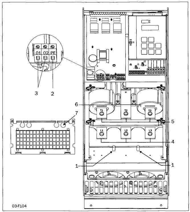
Fig. 21 Connection of MSF-170 to MSF-250.
