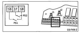
Fig. 67 Connection of external control inputs.
