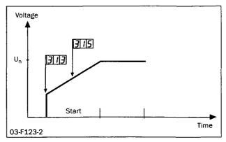
Fig. 39 Menu numbers for initial voltage and start time.
