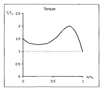
Fig. 3 Typical torque characteristics for the DOL start
