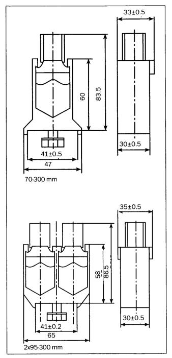
Fig. 72 The terminal clamp.
