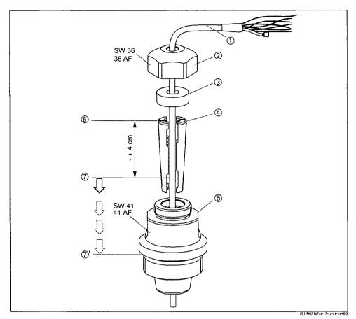
Fig. 6: Installing the Waterpilot FMX167 with cable mounting screw, here depicted with G I 1/2 thread
