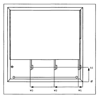
Fig. 16 Busbar distances MSF-310 to MSF-835.
