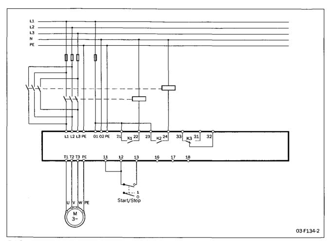
Fig. 45 Reverse current brake wiring example.
