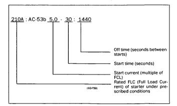
Fig. 29 AC53b rating example.
