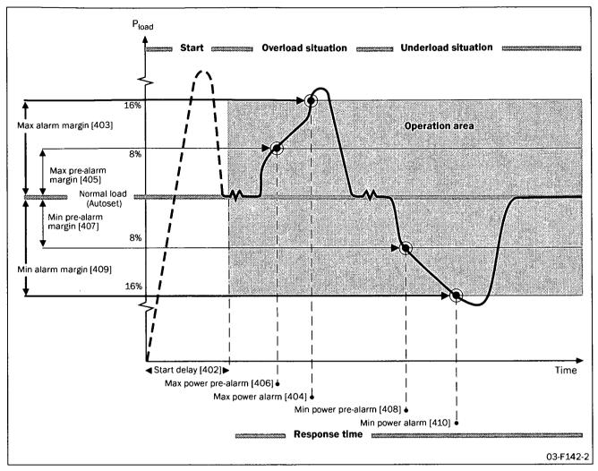
Fig. 52 Load monitor alarm functions
