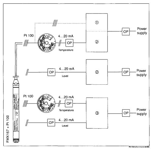
Fig. 13: Wiring up the measuring unit
