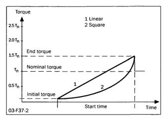
Fig. 37 Torque control at start
