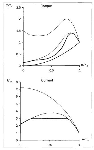
Fig. 9 Soft starting - voltage ramp with current limit
