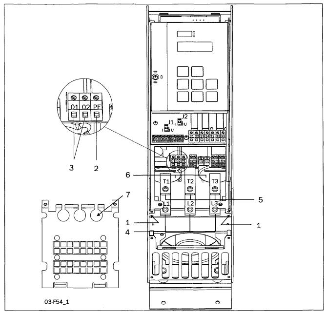
Fig. 19 Connection of MSF-017 to MSF-085.
