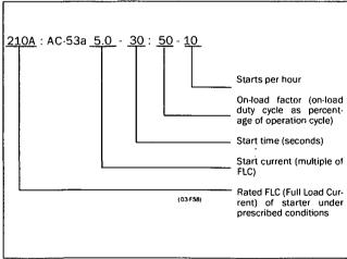
Fig. 27 AC53a rating example.
