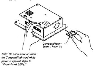
Information stored on a CompactFlash card by a G306A can be read by a card reader attached to a PC. This information is stored in IBM (Windows<sup>®</sup>) PC compatible FAT16 file format.
