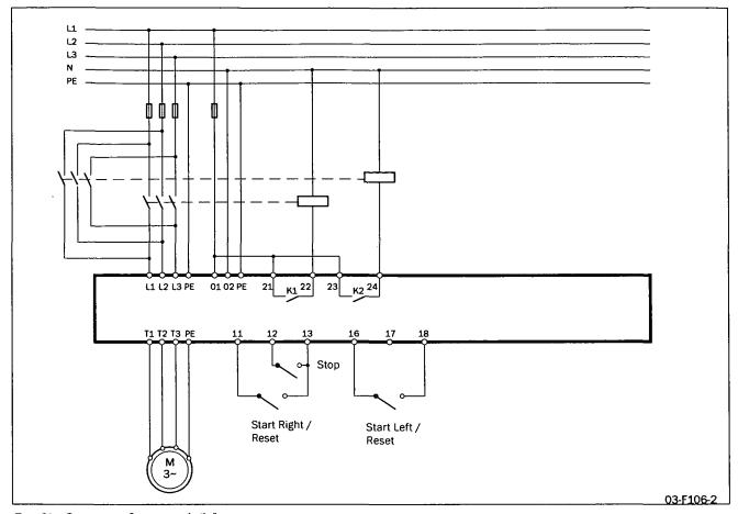
Fig. 65 Connection for start right/left
