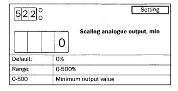
NOTE: The minimum value for scaling the analogue output is reset to the default value 0% if a new output value is chosen in menu [521].
