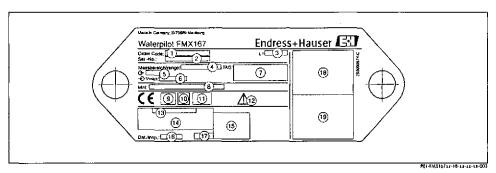
Fig. 1: Nameplate for Waterpilot FMX167
