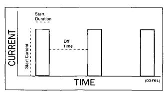
Fig. 30 Duty cycle, bypassed
