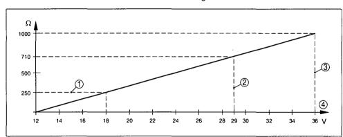
Fig. 10: Voltage diagram VEGABAR 74
