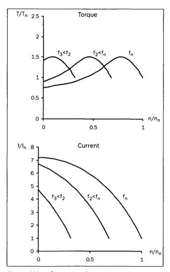
Fig. 12 Voltage/frequency regulation
