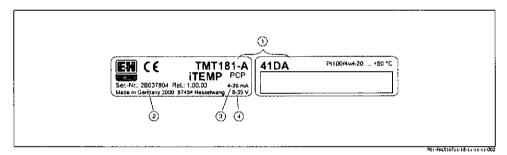
Fig. 3: Nameplate of temperature transmitter TMT181
