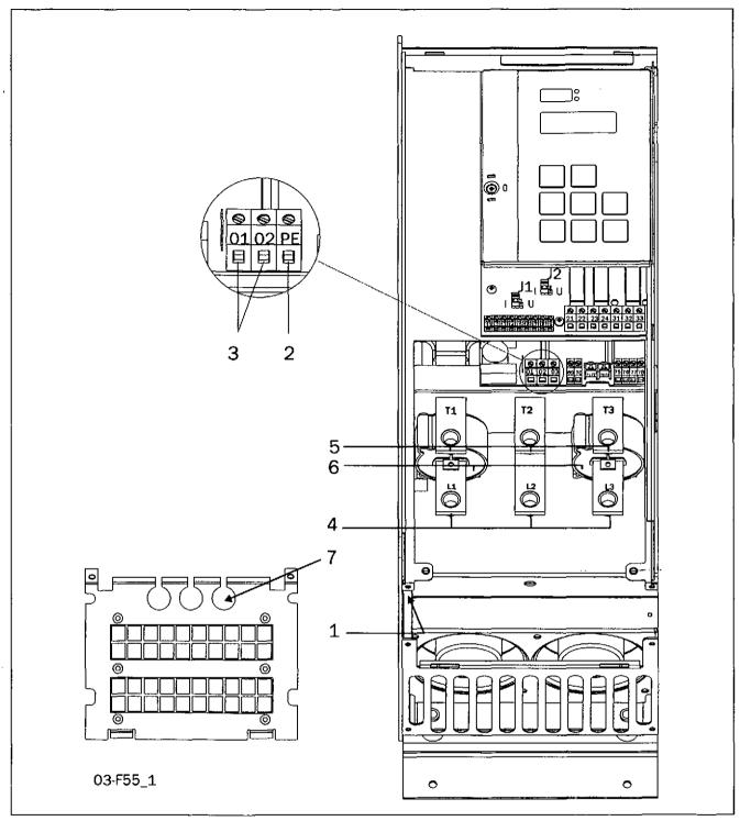
Fig. 20 Connection of MSF-110 to MSF-145.
