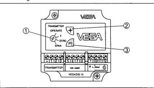
Fig. 7: Adjustment elements of VEGADIS 12
