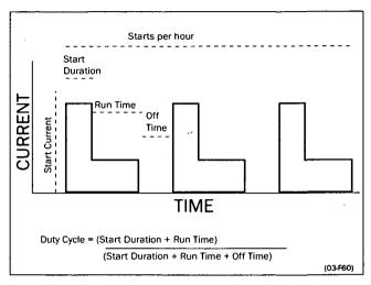
Fig. 28 Duty cycle, non-bypass.
