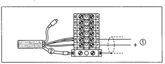
Fig. 5: Terminal assignment VEGABAR 74
