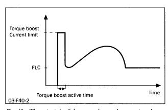
Fig. 42 The principle of the torque boost when starting the motor.
