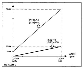
Fig. 60 Scaling of analogue output
