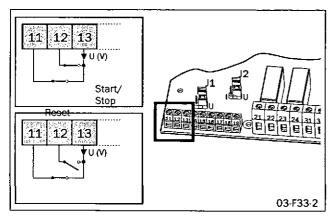
Fig. 63 2-wire connection of terminals for start/stop/separate reset
