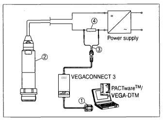
Fig. 8: Connecting the PC to the signal cable
