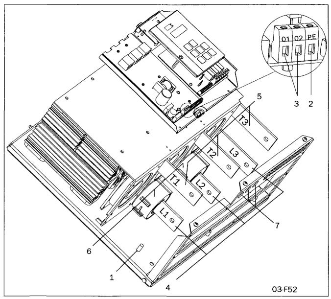
Fig. 22 Connection of MSF-310 to MSF-1400.
