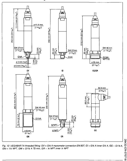
Fig. 12: VEGABAR 74 threaded fitting: GV = G% A manometer connection EN 837, GI = G% A inner G% A, GG = G1% A, GN = 1% NPT, GM = G1% A 70 mm, GR = % NPT inner % NPT
