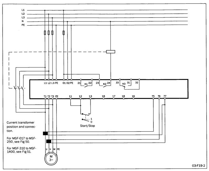
Fig. 49 Bypass wiring example MSF 310-1400.
