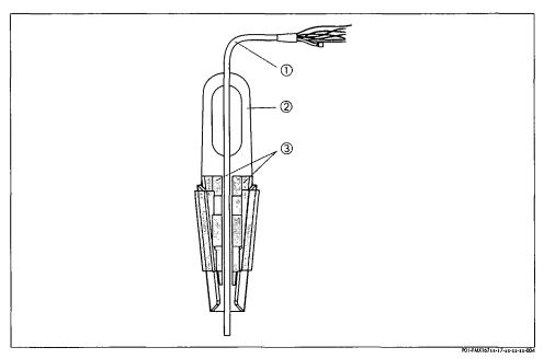
Fig. 5: Installing Waterpilot FMX167 with a mounting clamp
