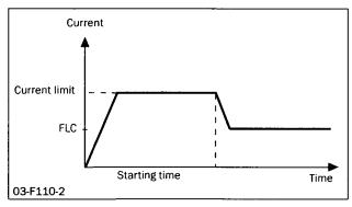
Fig. 41 Direct on-line start in combination with current limit
