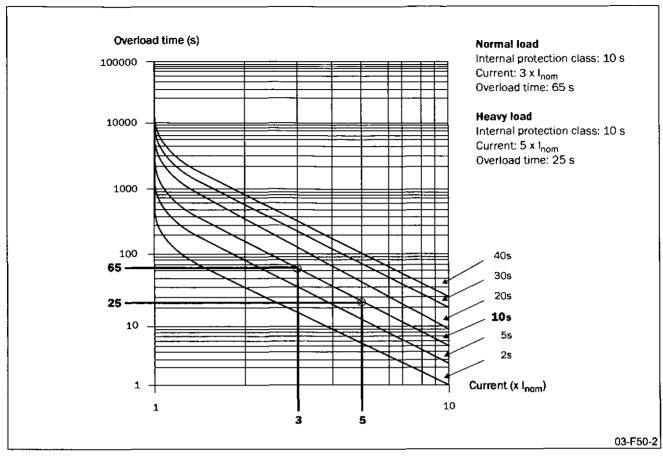
Fig. 34 The thermal curve
