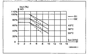
Illustration 10.6: Derating of I<sub>out</sub> for different T<sub>AMB, MAX</sub> for enclosure B, using SFAVM in Normal torque mode (110% over torque)
