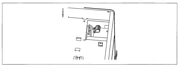
Illustration 5.40: Terminals for relay connections for C3 and C4. Located in the upper right corner of the frequency converter.
