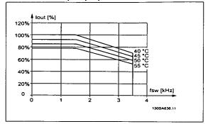
Illustration 10.18: Derating of  $I_{\text{Out}}$  for different  $T_{\text{AMB}, \text{MAX}}$  for enclosure E at 600 V, using SFAVM in Normal torque mode (110% over torque).
