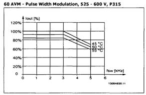
Illustration 10.13: Derating of Iout for different Tamb, max for enclosure D at 600 V, using 60 AVM in Normal torque mode (110% over torque). Note: P315 only.
