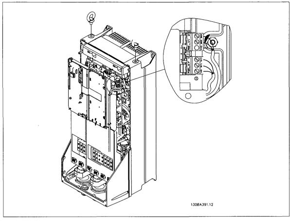
Illustration 5.37: Terminals for relay connection (C1 and C2 enclosures).
