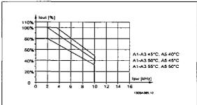
Illustration 10.2: Derating of  $I_{\text{Out}}$  for different TAMB, MAX for enclosure A, using SFAVM
