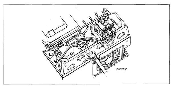
Illustration 5.11: How to connect to mains and earthing with mains disconnect switch.
