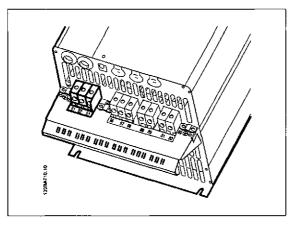
Illustration 5.17: How to connect C3 to mains and earthing.
