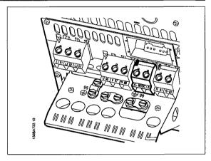
Illustration 5.30: DC bus connections for enclosure B4.
