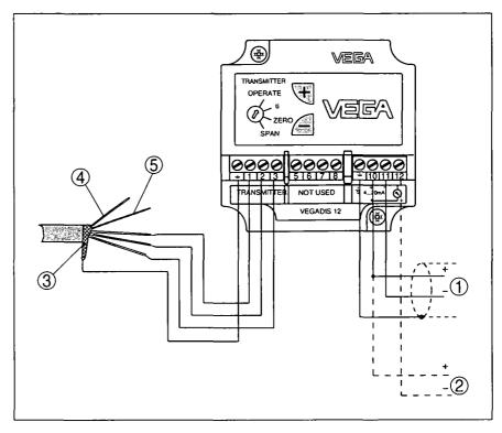
Fig. 6: Terminal assignment, VEGADIS 12
