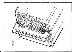
Illustration 5.35: Brake connection terminal for C3.
