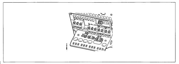
Illustration 5.39: Terminals for relay connections for B4.
