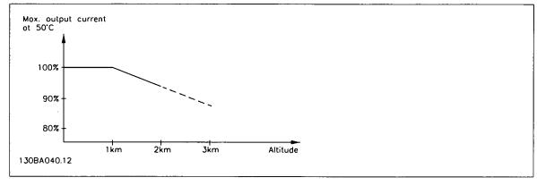
Illustration 10.19: Derating of output current versus altitude at TAMB, MAX. By altitudes above 2 km, please contact Danfoss regarding PELV.
