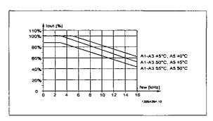
Illustration 10.3: Derating of  $I_{\text{out}}$  for different  $T_{\text{AMB}, \text{ MAX}}$  for enclosure A, using 60 AVM and maximum 10 m motor cable
