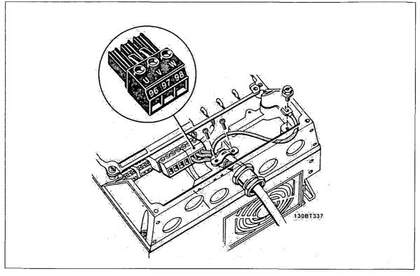
Illustration 5.22: First terminate the motor earth, then place motor U, V and W wires in terminal and tighten. Please ensure that the outer insulation of the motor cable is removed under the EMC clamp.
