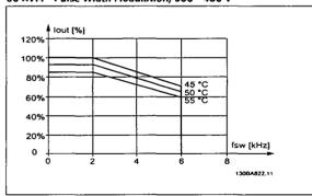
Illustration 10.15: Derating of Iout for different TAMB, MAX for enclosure E at 480 V, using 60 AVM in Normal torque mode (110% over torque)
