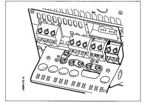
Illustration 5.34: Brake connection terminal for B4.
