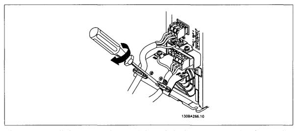
Illustration 5.21: Mount cable clamp to ensure 360 degree connection between chassis and screen, note the outer insulation of the motor cable is removed under the clamp.
