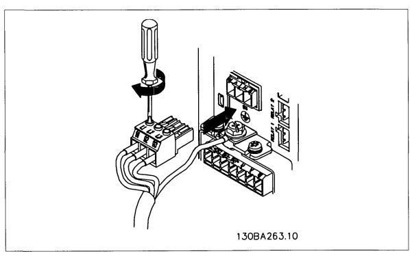
Illustration 5.8: Then mount mains plug and tighten wires.
