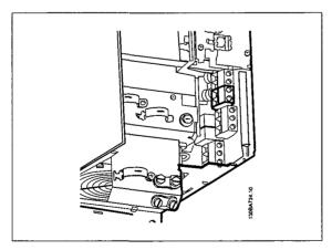
Illustration 5.33: Brake connection terminal for B3.
