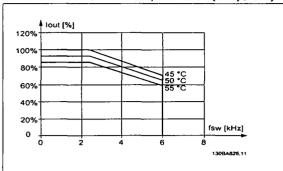
Illustration 10.11: Derating of  $I_{\text{out}}$  for different  $T_{\text{AMB, MAX}}$  for enclosure D at 600 V, using 60 AVM in Normal torque mode (110% over torque). Note: not valid for P315.
