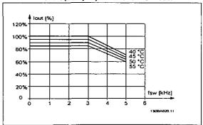
Illustration 10.10: Derating of I<sub>out</sub> for different T<sub>AMB, MAX</sub> for enclosure D at 480 V, using SFAVM in Normal torque mode (110% over torque)
