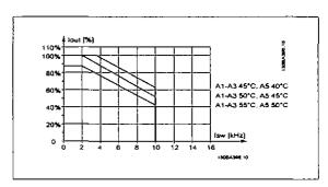
Illustration 10.4: Derating of  $I_{\text{Out}}$  for different  $T_{\text{AMB}, \text{MAX}}$  for enclosure A, using SFAVM and maximum 10 m motor cable
