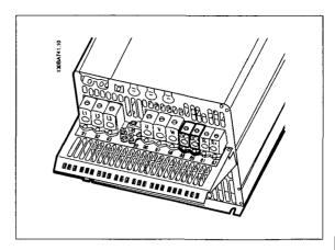
Illustration 5.32: DC bus connections for enclosure enclosure C4.
