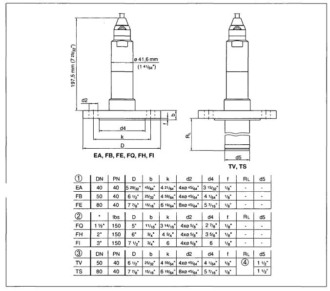
Fig. 15: VEGABAR 74 - flange connection
