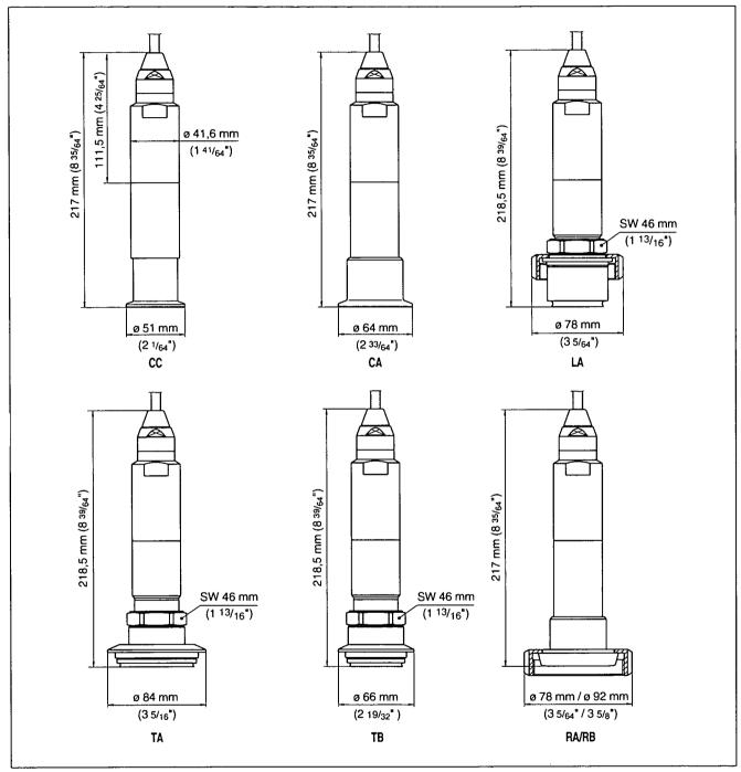
Fig. 13: VEGABAR 74 hygienic fitting:  $CC = Tri-Clamp \ 1\frac{1}{2}$ ",  $CA = Tri-Clamp \ 2$ ",  $LA = hygienic fitting with compression nut F40, <math>TA = Tuchenhagen \ Varivent \ DN \ 25$ ,  $RA/RB = bolting \ DN \ 40/DN \ 50$  according to DIN \ 11851
