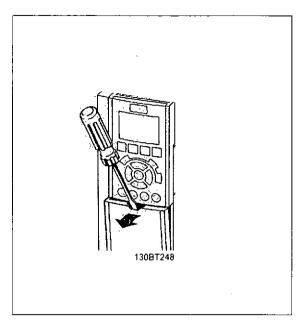
Illustration 5.41: Access to control terminals for A2, A3, B3, B4, C3 and C4 enclosures
