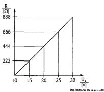
Load chart FMX167 for estimating load resistance. Subtract the additional resistances, e.g. resistance of extension cable, from the calculated value as shown in the equation.
