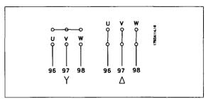
Illustration 5.19: Terminals for motor connection
