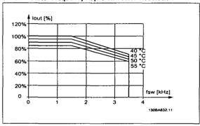
Illustration 10.14: Derating of  $I_{\text{out}}$  for different  $T_{\text{AMB, MAX}}$  for enclosure D at 600 V, using SFAVM in Normal torque mode (110% over torque). Note: P315 only.
