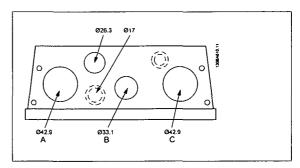
Illustration 5.2: Cable entry holes for enclosure 82. The suggested use of the holes are purely recommendations and other solutions are possible.
