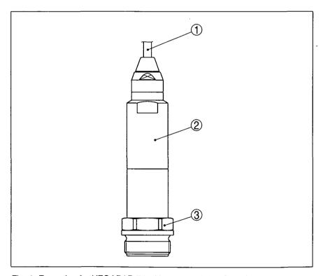
Fig. 1: Example of a VEGABAR 74 with process fitting G11/2 A
