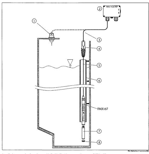
Installation examples, here shown with FMX167 with an outer diameter = 0.87 in (22 mm)
