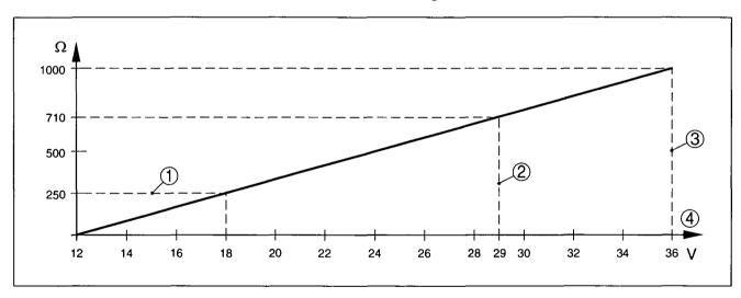
Fig. 10: Voltage diagram VEGABAR 74
