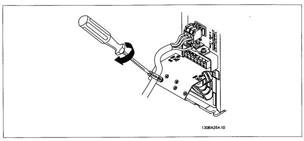
Illustration 5.9: Finally tighten support bracket on mains wires.
