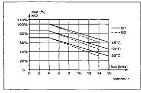
Illustration 10.5: Derating of  $I_{\text{Out}}$  for different  $T_{\text{AMB}, \text{MAX}}$  for enclosure B, using 60 AVM in Normal torque mode (110% over torque)
