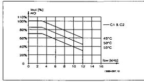
Illustration 10.7: Derating of low for different TAMB, MAX for enclosure C, using 60 AVM in Normal torque mode (110% over torque)
