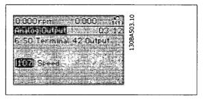
Illustration 8.8: Step 7: Use the up/down navigation keys to select between the different choices. Press [OK].
