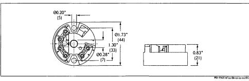
Temperature transmitter TMT181 (4 to 20 mA), dimensions in inches (mm)
