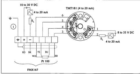
FMX167 with Pt 100 and TMT181 temperature transmitter (4 to 20 mA), version "5" for Feature 70 in the order code (→ see Page 18).
