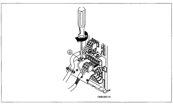
Illustration 5.20: First terminate the motor earth, then place motor U, V and W wires in plug and tighten.
