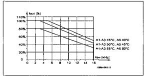
Illustration 10.1: Derating of  $I_{\text{out}}$  for different  $T_{\text{AMB, MAX}}$  for enclosure A, using 60 AVM
