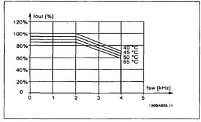
Illustration 10.12: Denating of  $I_{\text{out}}$  for different  $T_{\text{AMB, MAX}}$  for enclosure D at 600 V, using SFAVM in Normal torque mode (110% over torque). Note: not valid for P315.
