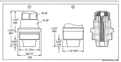
Extension cable mounting screws, dimensions in inches (mm) Order number: 52009311
