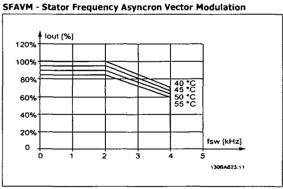
Illustration 10.16: Derating of Iout for different TAMB, MAX for enclosure E at 480 V, using SFAVM in Normal torque mode (110% over torque)
