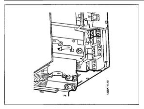
Illustration 5.29: DC bus connections for enclosure B3.
