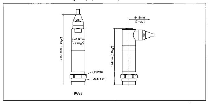
Fig. 16: VEGABAR 74 - connection for paper industry: BA/BB = M44x1.25
