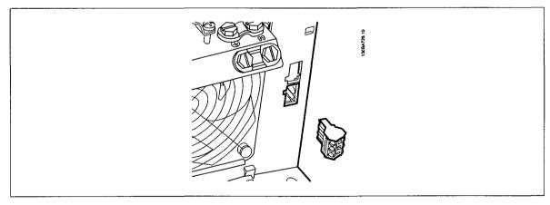
Illustration 5.38: Terminals for relay connections for B3. Only one knock-out is fitted from the factory.
