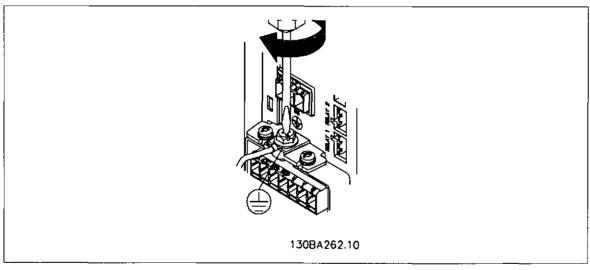
Illustration 5.7: When mounting cables, first mount and tighten earth cable.
