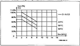
Illustration 10.8: Denating of  $I_{\text{out}}$  for different  $T_{\text{AMB}, \text{ MAX}}$  for enclosure C, using SFAVM in Normal torque mode (110% over torque)
