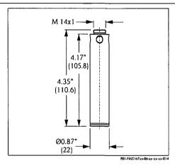
To prevent sideways movement leading to measuring errors or to ensure that the device lowers into a guide tube, Endress+Hauser provides additional weights.
