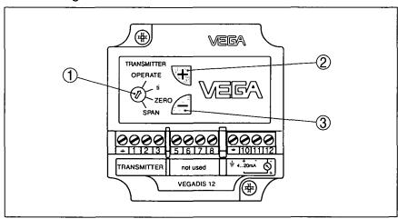
Fig. 7: Adjustment elements of VEGADIS 12
