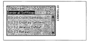
Illustration 8.6: Step 5: Use the up/down navigation keys to scroll down to i.e. 03-12 *Analog Outputs*. Press [OK].
