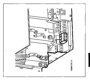
Illustration 5.13: How to connect to mains and earthing for 83 without RFI.
