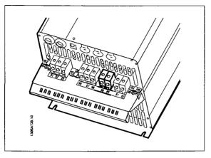
Illustration 5.31: DC bus connections for enclosure C3.
