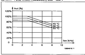
Illustration 10.9: Derating of  $I_{\text{OM}}$  for different  $T_{\text{AMB, MAX}}$  for enclosure D at 480 V, using 60 AVM in Normal torque mode (110% over torque)
