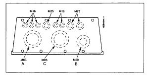
Illustration 5.4: Cable entry holes for enclosure C2. The suggested use of the holes are purely recommendations and other solutions are possible.
