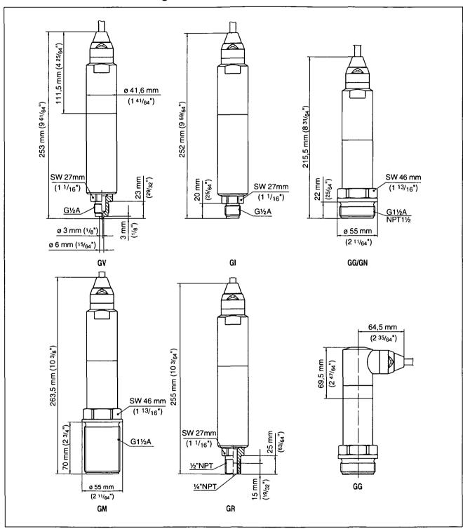
Fig. 12: VEGABAR 74 threaded fitting: GV = G% A manometer connection EN 837, GI = G% A inner G% A, GG = G1% A, GN = 1% NPT, GM = G1% A 70 mm, GR = % NPT inner % NPT
