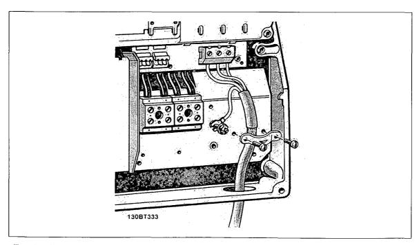
Illustration 5.23: First terminate the motor earth, then Place motor U, V and W wires in terminal and tighten. Please ensure that the outer insulation of the motor cable is removed under the EMC clamp.
