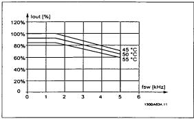
Illustration 10.17: Derating of  $I_{\text{Out}}$  for different  $T_{\text{AMB, MAX}}$  for enclosure E at 600 V, using 60 AVM in Normal torque mode (110% over torque).
